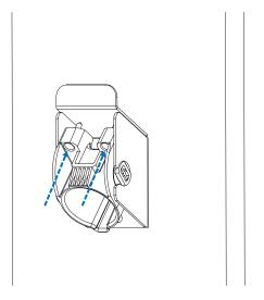
Figure 2-15 Secure the hook
