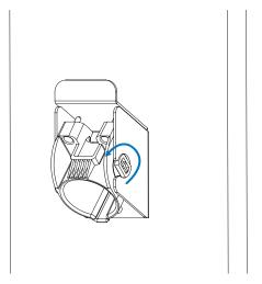
Figure 2-14 Rotate the holster
