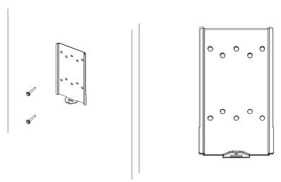
Figure 2-1 Fasten mounting bracket
