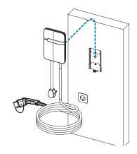
Figure 2-3 NC7000 Series Charger and mounting bracket
