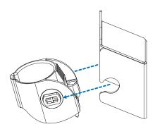
Figure 2-11 Separate the holster
