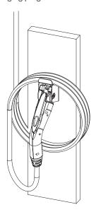
Figure 2-16 Place NC7000 series charging plug.
