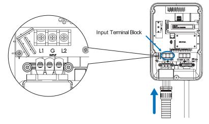
Figure 2-10 Input wiring
