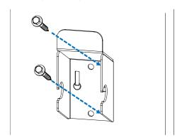
Figure 2-12 Secure the hook
