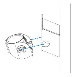
Figure 2-13 Secure the holster
