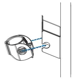
Figure 2-13 Secure the holster
