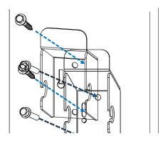
Figure 2-12 Secure the hook
