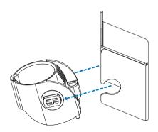
Figure 2-11 Separate the holster
