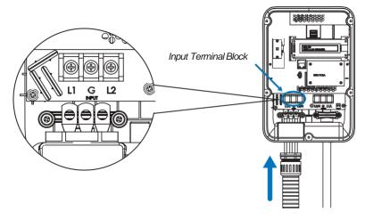
Figure 2-10 Input wiring
